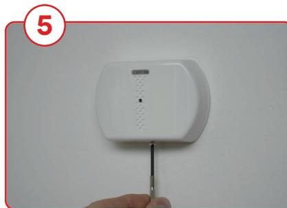
5 Use the tiny screw that is included to secure the cover to the backplate on the bottom of the device.
