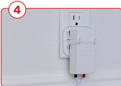
Use your wire tie to hold the power adaptor in place. You can clip off any excess wire afterward.
