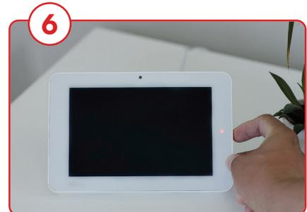
Take your panel, and push and hold the standby button on the side for 3 seconds to power it up.
