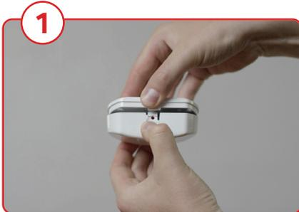
1 Remove your sensor from its backplate by pressing open the tab at the bottom.
