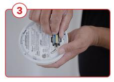
Insert the battery provided into the carbon monoxide detector.
