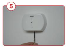
Use the tiny screw that is included to secure the cover to the backplate on the bottom of the device.
