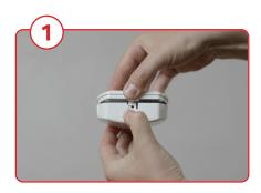
Remove your sensor from its backplate by pressing open the tab at the bottom.
